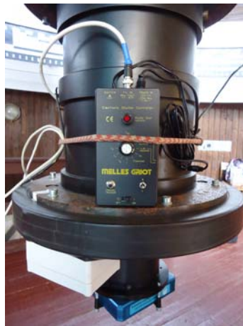
Figure 19. Electronic Shutter Melles Griot 43 mm.
