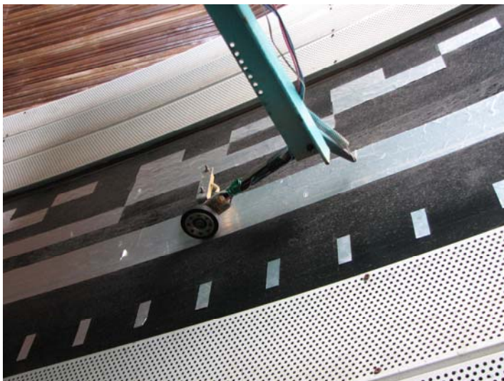
Figure 25. Magnetic detector designed by R. Janulis for the dome synchronization (Foto: R. Janulis).
