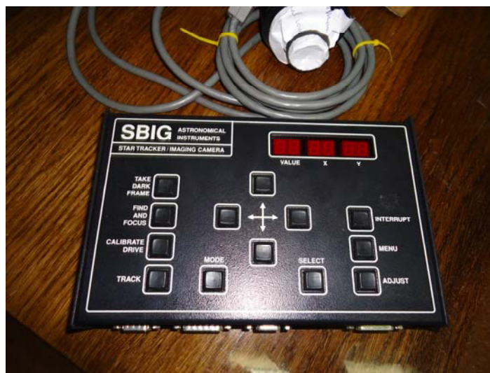
Figure 23. Star Tracker/Imaging camera. "Santa Barbara Instrument Group" (SBIG) CCD camera autoguider
