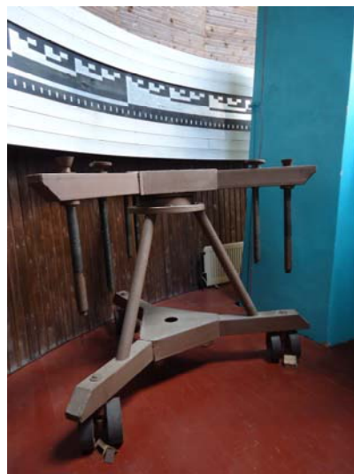
Fig. 12. Cleaning table for the mirror of 1.65 m.
