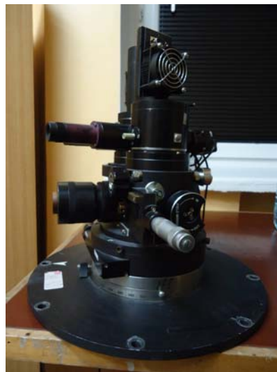
Figure 7. Three-channel high Speed CCD photometer.
