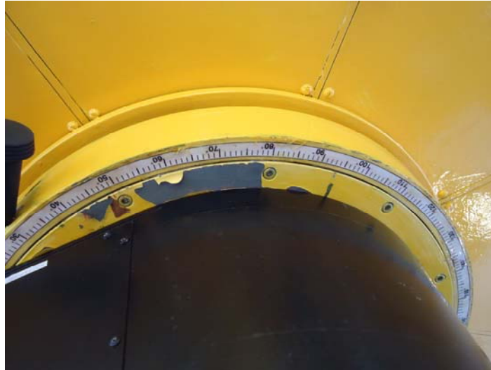
Figure 26. Derotator (scale in degrees).
